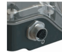
Art.Nr. 49894036 - Solenoid valve connection with 380 mm cable, in box soldered and carried out by a second gland M16x1,5 mm - M12 plug connection, 5-pole
